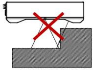
Do not install the sensor near objects that might occlude a camera's view of the light
