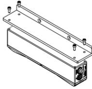
Mount the sensor using four M5 x 0.8 screws of suitable length. The recommended thread engagement into the housing is 8 - 10 mm.
