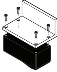
Mount the sensor using four M5 x 0.8 screws of suitable length. The recommended thread engagement into the housing is 8 - 10 mm.
