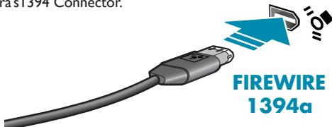
**NOTE:** The camera relies on the 6-pin 1394 cable to provide power. If using an interface card other than that provided, ensure that adequate power is provided.
