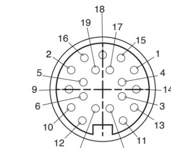
View: Looking into the connector on the sensor.
