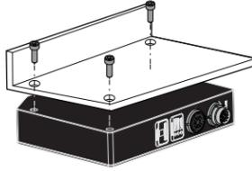
Mount the sensor using four M6 x 1.0 screws of suitable length. The recommended thread engagement into the housing is 8 - 10 mm.
