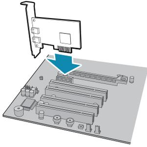
Ensure the card is installed per the manufacturer's instructions. Alternatively, use your PC's built-in host controller, if equipped.
